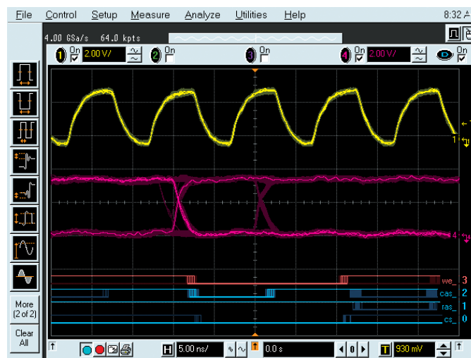
Figure 2: Six-channel measurement: Data line during a write trigger on RAS, CAS, WE, CS and CLK.
